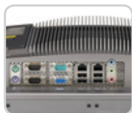
Rich standard I/O support and dual LAN
